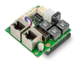
The new *EPOS4* Compact 50/5 EtherCAT ©maxon motor ag (56.5 x 55.0 x 31.9 mm)
